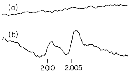
Figure 2. Optically-generated ESR signal in single-crystal silicon etched in \text{HNO}_3 -HF-HAc with reformed native oxide: (a) light off, (b) light on
